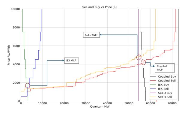
Figure 5 IEX, SCED and Market Coupling Illustrative Example 1: MCP < SMP
